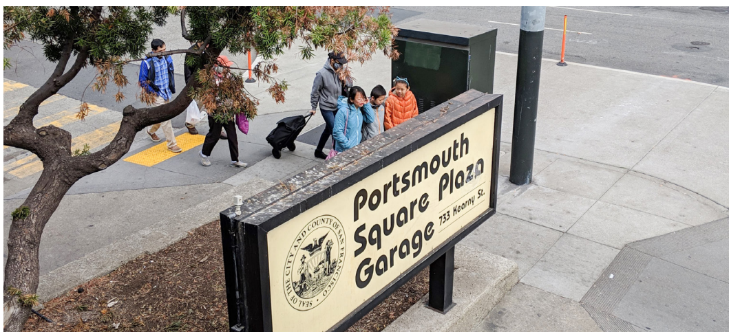
Figure 23. Garage Sign and Utility Cabinet Create a Pinch Point Between the Entry and Exit Driveways
