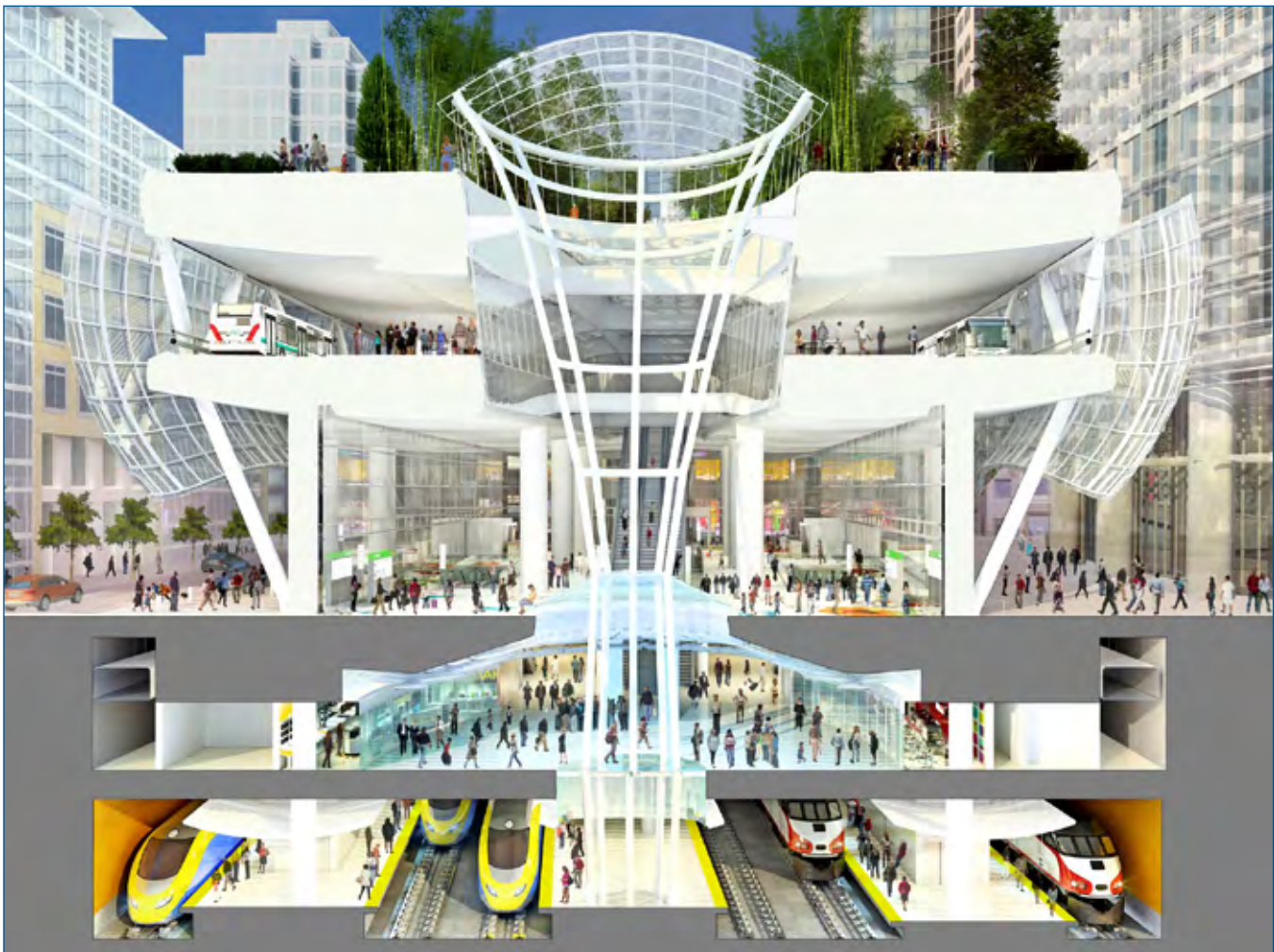
The Salesforce Transit Center, pictured above, officially opened July 2019. The structure includes a two-level trainbox—funded in part from $400 million in American Reinvestment and Recovery Act funds—which will house the future train station mezzanine and the train platform.
